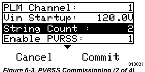
Figure 6-3. PVRSS Commissioning (2 of 4)
