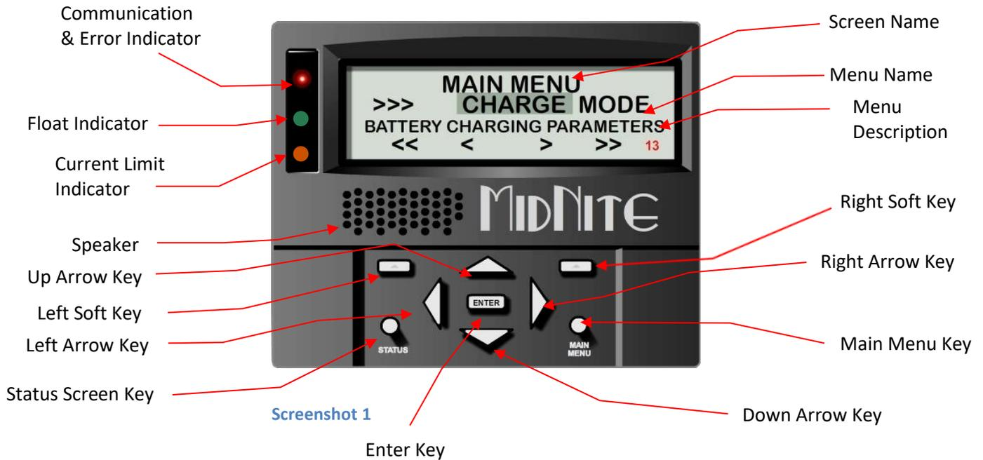
Most settings can be accessed and modified. Navigate using the LEFT & RIGHT arrows. Pressing ENTER takes you into that menu. The MAIN MENU key also backs you out of any submenu. Use the soft-keys for options & views. Be sure to press ENTER to save changes before backing out of any menu/submenu.
