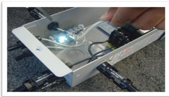
Figure 18 – Actual Arc Fault
