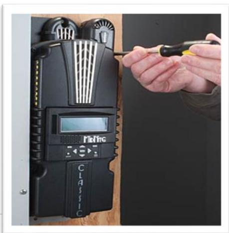
Remove the four screws holding the front cover of the Classic charge controller (see Figure 27).
