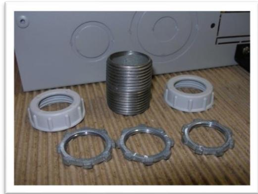
Figure 5 – Nipple, locknuts, and bushings
