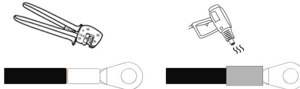
**Figure 4-15 Crimp and Seal Lugs**
