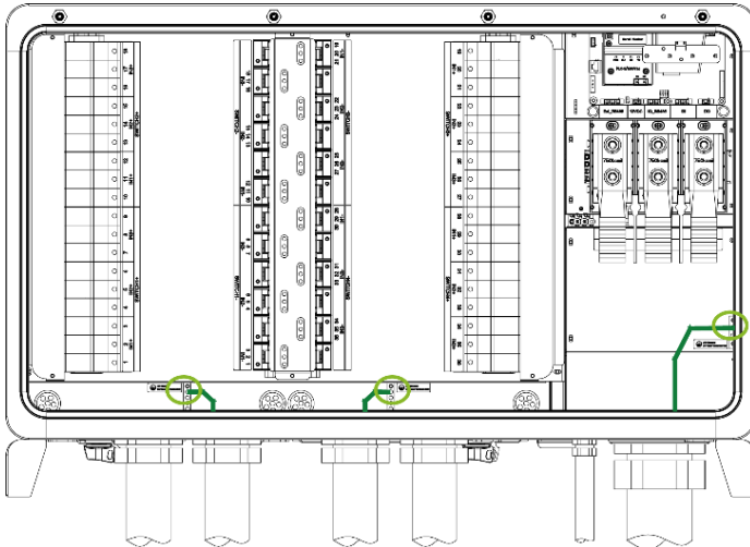
Figure 4-4 Internal DC and AC Ground Terminals
