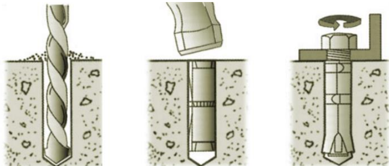
Figure 3-8 Drill Holes, Set Anchors, and Tighten Assembling Bolts
