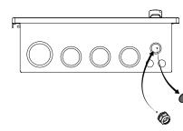
Starting with the far right conduit hole, install conduit fittings (suitable for desired ingress rating).
