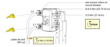
4 Connect grounded service entrance cable/ground electrode, and bonding screw to neutral terminals.
