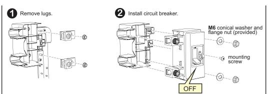
3 Connect L1/L2, and install Touch Safe Guards (see circuit breaker manual)
