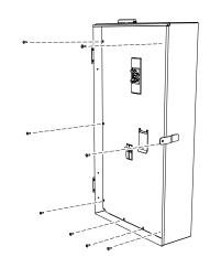
If needed, remove the cap and install a Square D Series B conduit hub (see table below).
