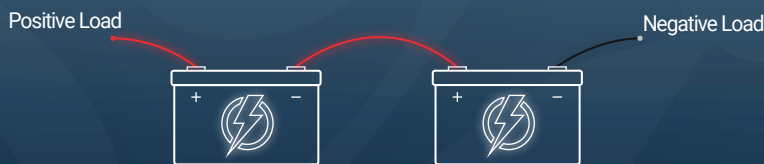
Series Connection 24V 270Ah Bank Increases Voltage, Ah stays the same.
