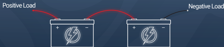
Series Connection 24V 270Ah Bank
