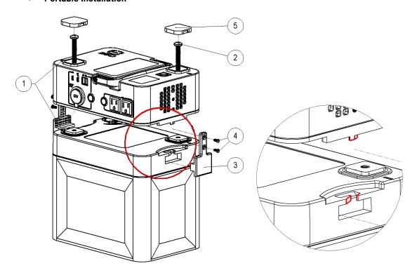
Before installation, make sure all the switches are in the OFF position (flush and LED off).
