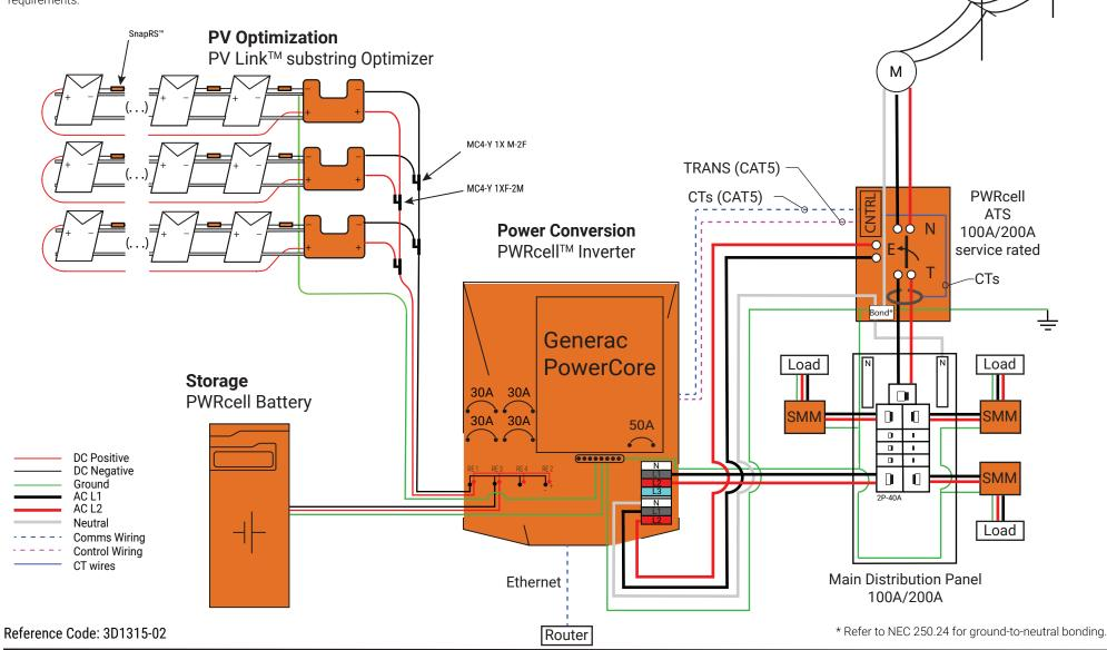
This design shows the Generac PWRcell Whole Home Backup solution. This solution allows for load management capability using Generac SMMs to shed 240V loads as needed.
