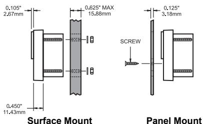
**Surface Mount:** Drill five clearance holes as shown below. The part number of the meter will determine the size and location of the clearance holes. Use the nuts and washers supplied in the accessory package to secure the four mounting studs to the mounting surface. This method will work on mounting surfaces up to 5/8" thick.
