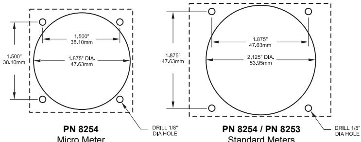
**Panel Mount:** For thicker mounting surfaces, the meter can be mounted into a 0.125" thick panel. Blue Sea Systems offers meter mounting panels for our standard size meters only. Use PN 8013 to mount a single meter or PN 8014 to mount two meters.
