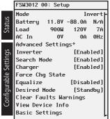
Figure 20 Device Setup Menu Screen
