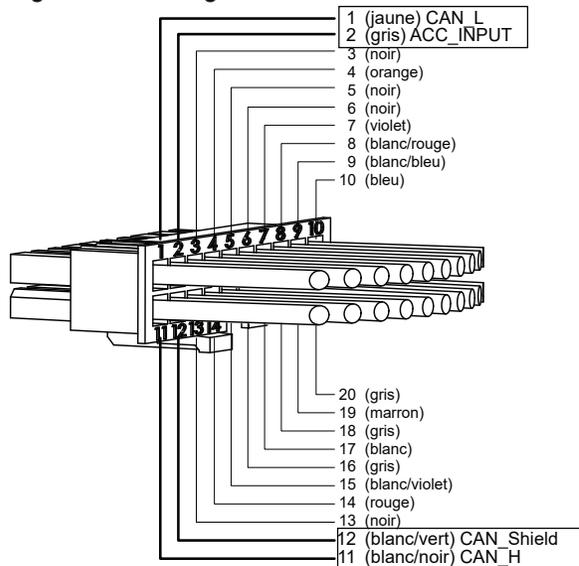
Figure 18 Port 20 broches CC Brochage des ports
