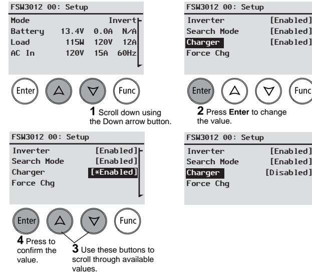
Figure 21 Selecting and Changing a Configurable Setting
