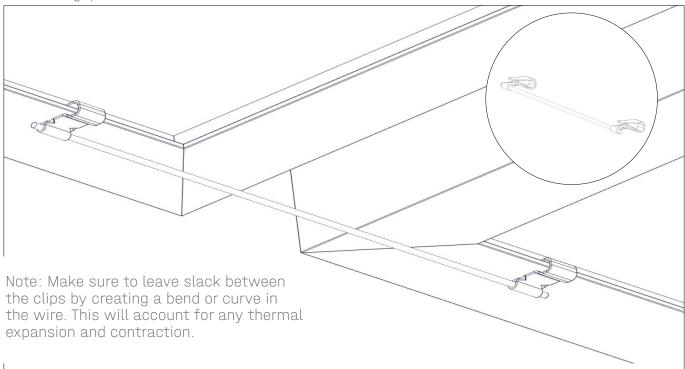
Dynobonds will also be used North and South connecting separate rows of modules. Only one connection point is needed to make a bridge from row to row. Installation of Dynobonds connecting rows can be done while installing modules, or on the outer edges of the array after installation is complete.
