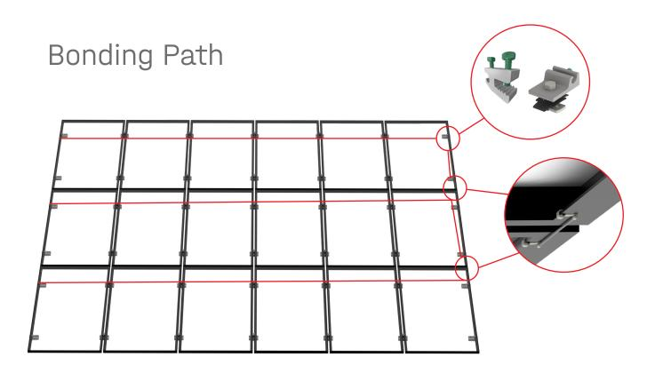
All K2 standard mid and end clamps are UL 2703 listed for bonding listed module frames. To ensure a proper system ground path, install Dynobond at each module row connection, see F1. Install equipment grounding conductor usisng either an Everest Ground Lug or an Ilsco Lug installed onto the MiniRail, see F2.
