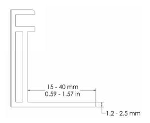
Frame Compatibility: Flange Thickness = 1.2 - 2.5 mm Flange Width = 15 - 40 mm
