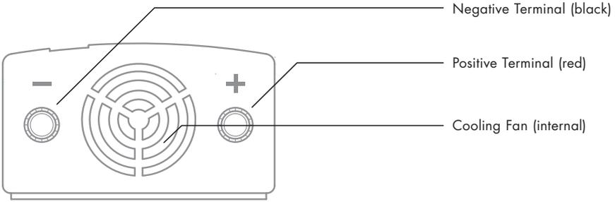
High Speed Fan – The fan turns on when there is a high load or an elevated temperature to keep the inverter cool. Do not block. Keep 2-inch clearance.
