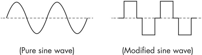
This modified sine wave has a root mean square (RMS) voltage of 115 volts. Most ordinary AC voltmeters are calibrated to read "average" voltage and assume that the AC waveform will be a pure sine wave. These meters will not correctly read MSW voltage, and will display about 20 to 30 volts too low. Any multi-meter identified as "TRUE RMS" will accurately read MSW correctly.
