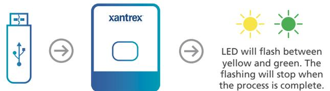
Insert the USB into the inverter/charger unit. Upon inserting the USB stick, the FREEDOM XC PRO inverter/charger LED should flash showing that the USB is recognized and the firmware is being downloaded.
