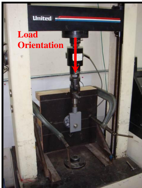
Figure 2a. Shear Perpendicular to Rafter
