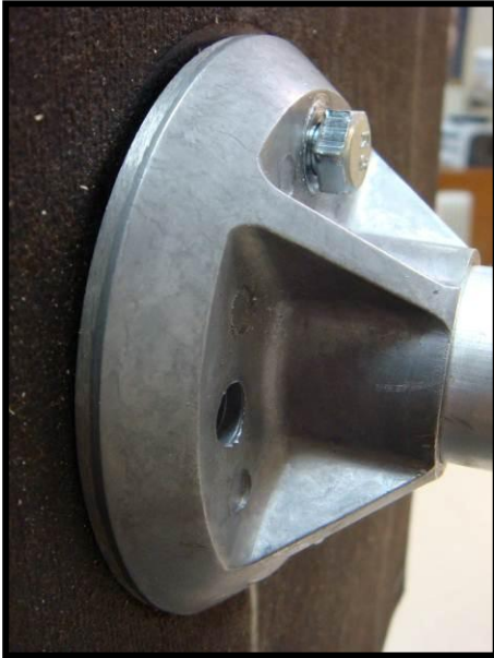
Figure 3. Lag Bolt Pull-Out Shear Parallel to Rafter
