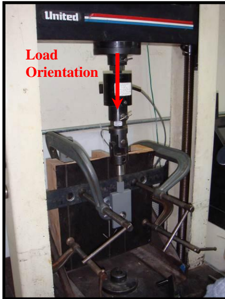
Figure 1a. Shear Parallel to Rafter
