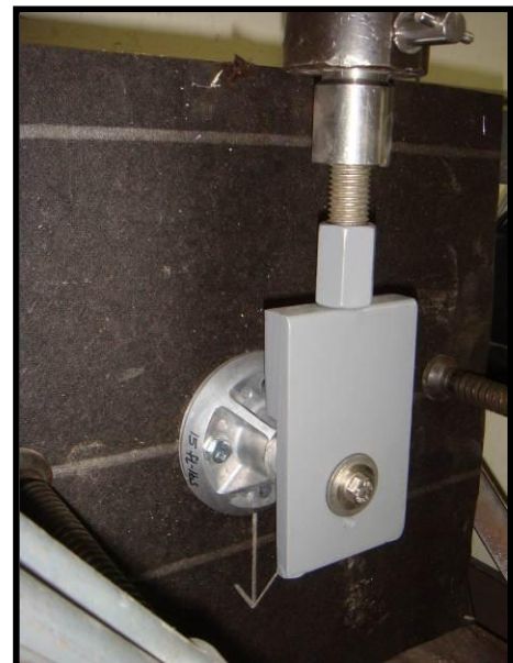
Figure 2b. Shear Test Close-up
