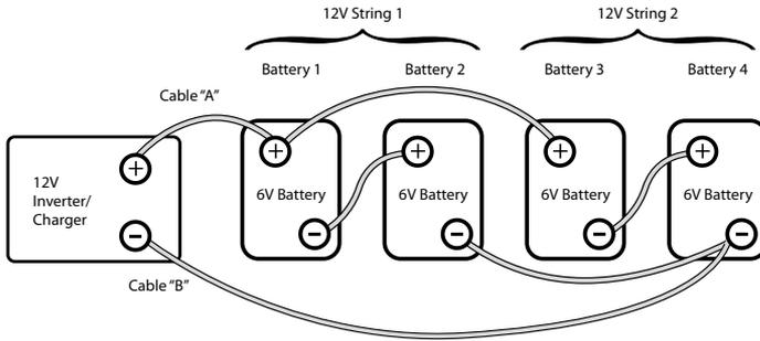
Fig. 4.4 Series-Parallel Connection
