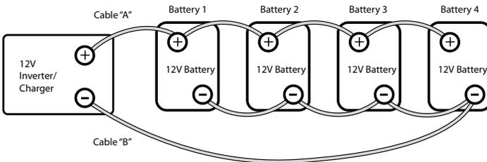
Fig. 4.3 Parallel Connection
