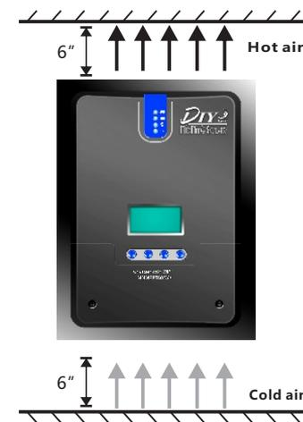
Fig. 2.1 Installation and heat dissipation
