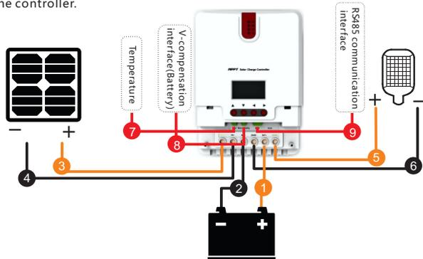
Fig. 2.3 Wiring sequence
