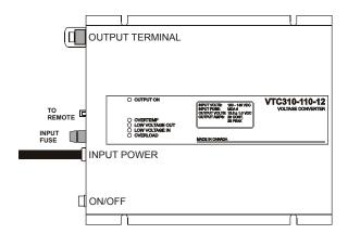
Allow at least 1 inch of clearance all around the case for cooling. The best mounting configuration is to mount the unit on a vertical surface oriented as shown. Use #10 screws of the appropriate type for the mounting surface to securely mount the unit.
