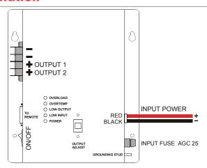
Allow at least 1 inch of clearance all around the case for cooling. The best mounting configuration is to mount the unit on a vertical surface oriented as shown. Use #10 screws of the appropriate type for the mounting surface to securely mount the unit.
