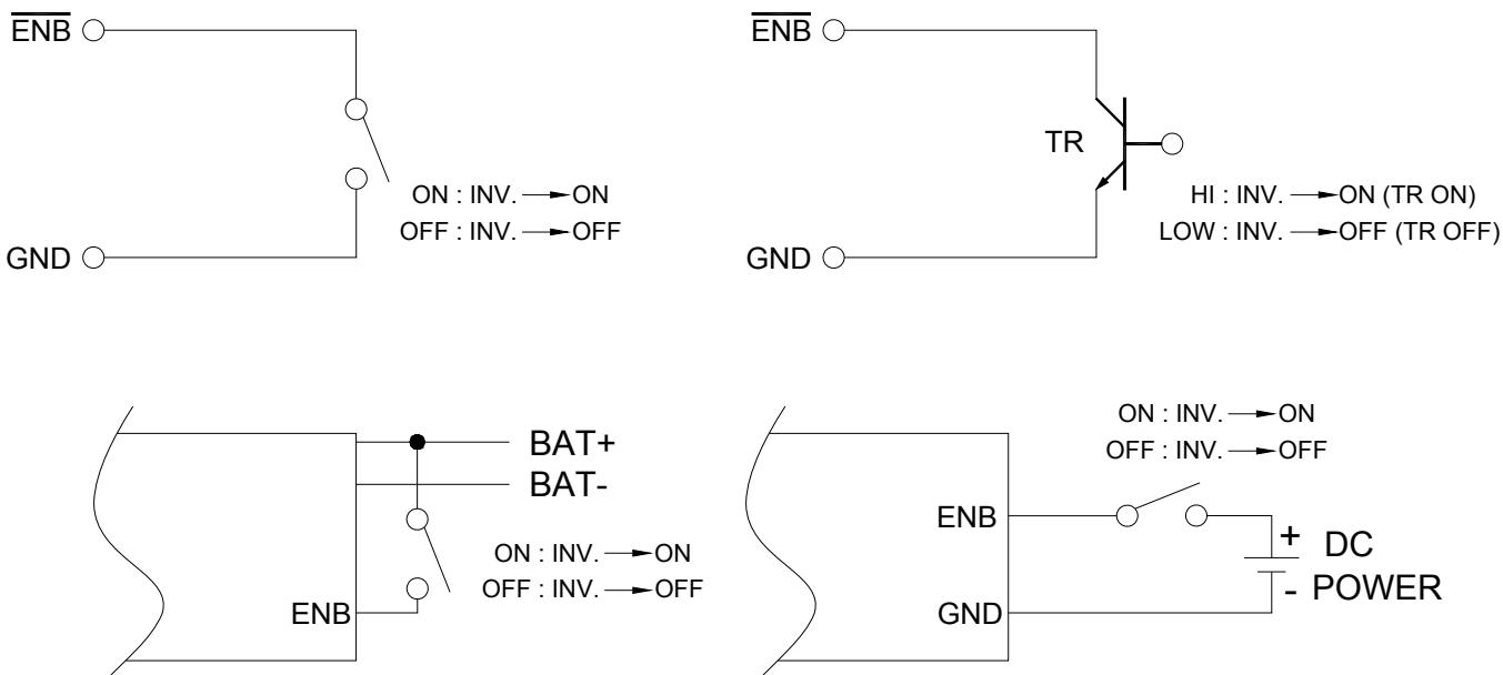
NOTE: At one time, only one remote function should be used to control the inverter.
