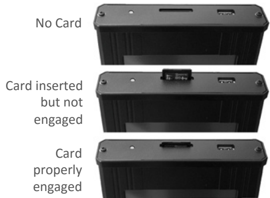
Figure 17: Insertion of the memory card
