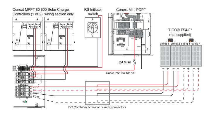
\*IMPORTANT: The Rapid Shutdown functionality is achieved only when the PV modules are equipped with compatible models of TIGO® TS4-F, installed according to local codes and standards. Other TS4 variants are not supported.
