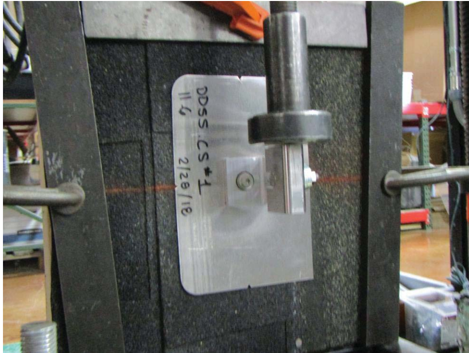
Photo 7: Lateral Perpendicular to Rafter Eccentric Load (pre-test) – Block Inside
