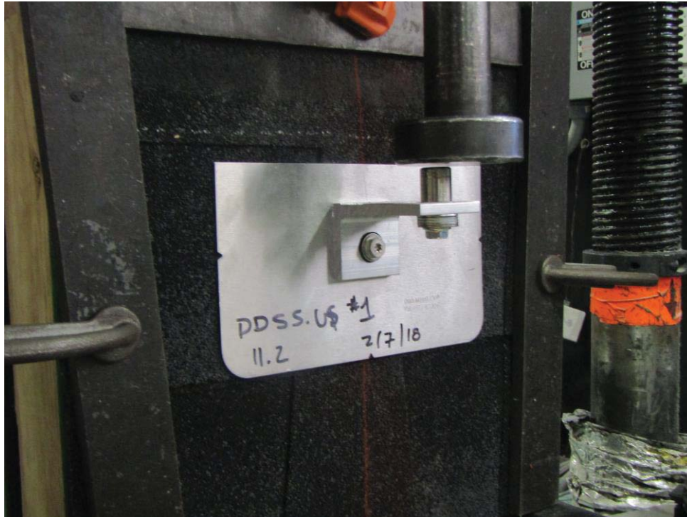
Photo 5: Lateral Parallel to Rafter Eccentric Load (pre-test) - Upslope
