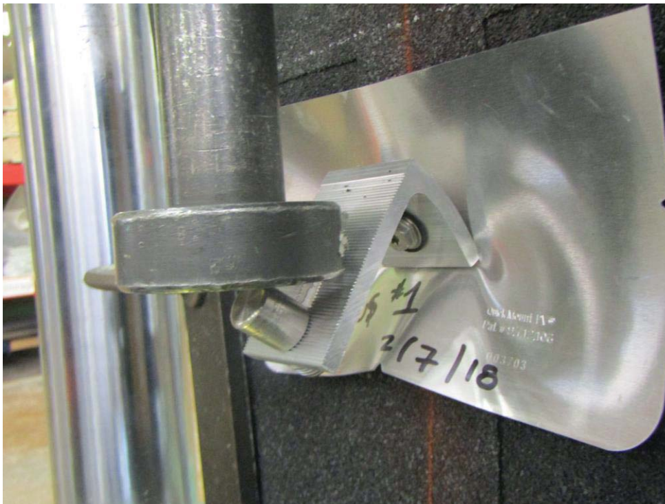
Photo 6: Lateral Parallel to Rafter Eccentric Load (post-test) - Upslope
