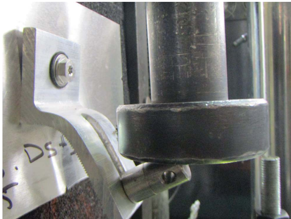
Photo 4: Lateral Parallel to Rafter Eccentric Load (post-test) - Downslope
