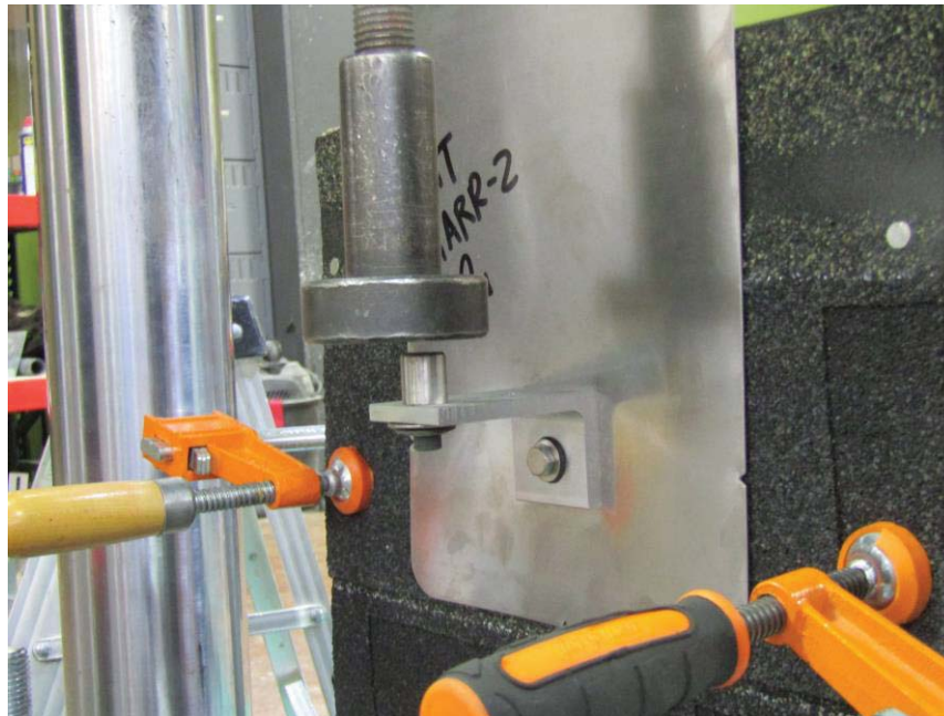
Photo 9: Lateral Parallel to Rafter Eccentric Load (pre-test) - Upslope
