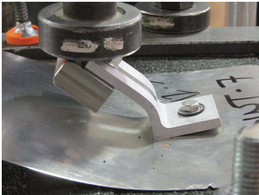
Photo 6: Compressive Load (Block with Teeth, post-test)
