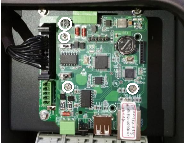
Figure 2.3 - Ethernet Network Card Installed
