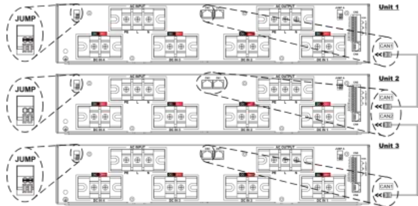
Figure 17-3. Parallel connection via jumper setting
