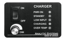
A remote control panel may be connected to the battery charger using a 9-pin D-connector that attaches to the side of the battery charger. The remote control panel and D connector are part of the remote control option. The remote control panel allows the unit to be operated remotely as well as duplicating all the diagnostic indicators and audible alarm.
