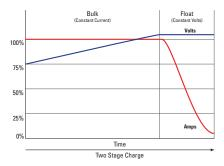
This charger features user selectable 2 or 3 stage charging. The charging profile is selected by moving the slide switch on the front panel up to 3 stage or down for 2 stage charging.
