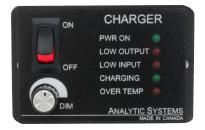
A remote control panel may be connected to the inverter using a 9-pin D-connector, which attaches to the battery charger. The remote control panel and D connector are part of the remote control option. The remote control panel allows the unit to be operated remotely as well as duplicating all the diagnostic indicators and audible alarm.
