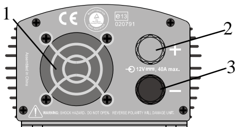
Figure 5 DC Panel on the XPower 300
