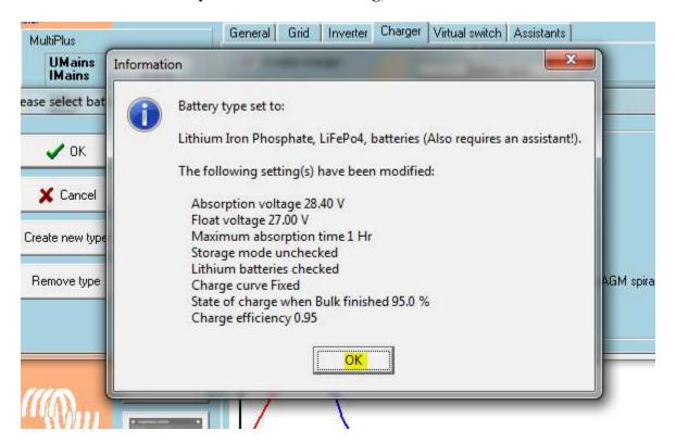
7. Back on the Charger tab make sure that "enable charger" and "lithium batteries" has a check mark. Then the "Charge curve" should say <u>Fixed</u>.
