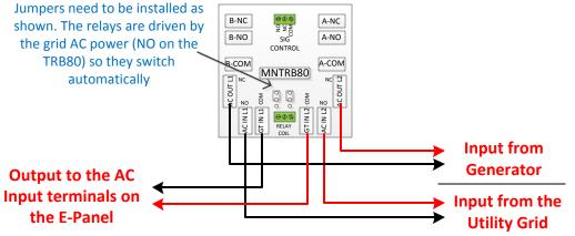
As shown utility in could be a second generator, The terminals (NO) that Utility in are connected to trigger the relay so these are the priority terminals.
