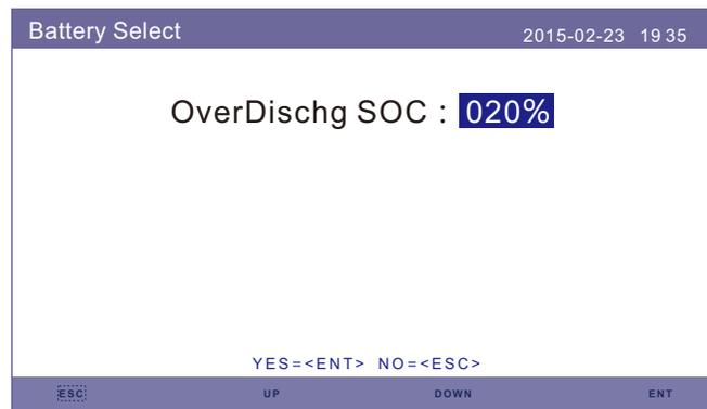
Figure 5.29 Over Discharge SOC.
