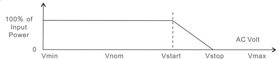
Figure 5.45 Volt-Watt characteristic
