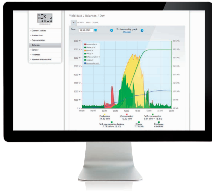
Daily overview: Surplus PV (in light green) is used to charge batteries for later use of the stored electricity, increasing self-consumption and reducing electricity bills
