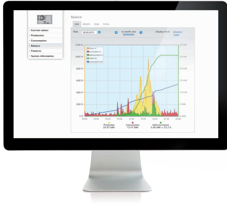
The smart Solar-Log® energy management controls, displays, and presents self-consumption of generated PV power, shown on the graph above in green.
