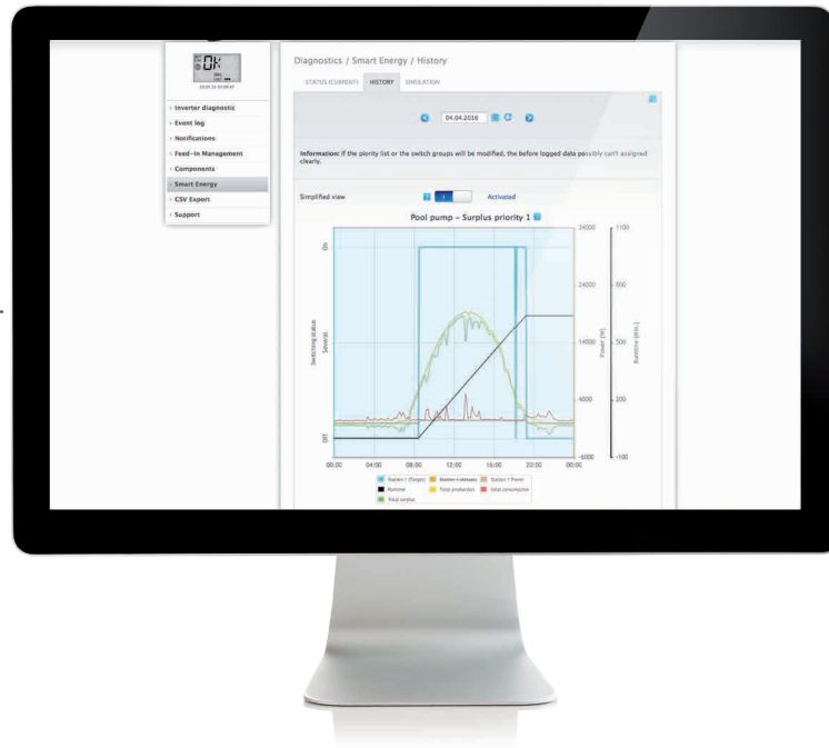
History: The configured Smart Energy profiles are visualized here. This provides a quick and easy way of checking configured settings.
