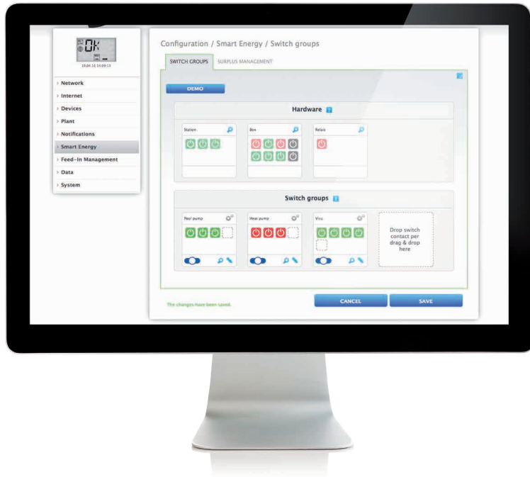
Smart Energy Configuration: Switching contacts can be added to switching groups and will be actively managed by the Solar-Log™.
