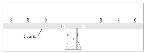
When installing the Rails orient their profiles as shown.
