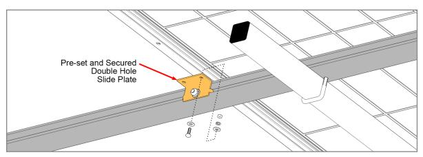
Align Module mounting holes with the installed Double Hole Slide Plates and secure Module with 1/4" x 3/4" Hex Bolt, Flat Washers, Lock Washer and Hex Nut. Finger tighten for now. Repeat on opposite Rail.
