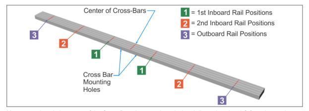
Measure and mark the center of the Cross-Bars then use the calculated dimensions I and O from the previous page to mark off their respective Rail positions. The image below shows these marks and their relationship to the Cross-Bars and Rails after assembly.
