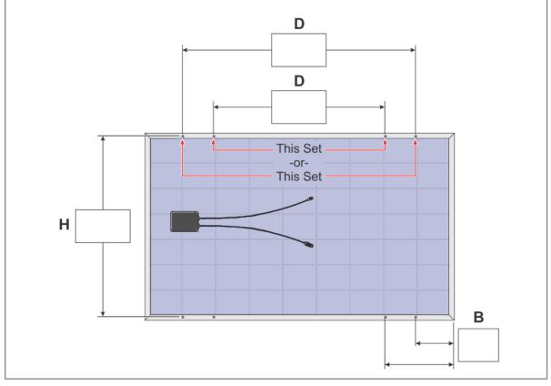
The dimensions must be taken from the site-specific Modules. The dimensions will be used to calculate the Module Rail positions.
