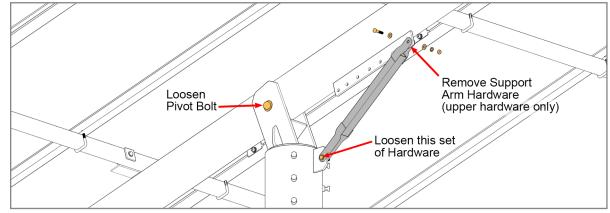
A. While one person holds the south edge of rack, the other loosens the Pivot Bolt and the hardware securing the lower end of the Support Arm hardware.
