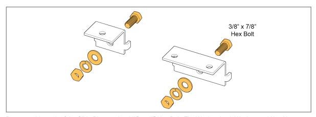
Pre-assemble each of the Slide Plates using 3/8" x 7/8" Hex Bolt, Flat Washer, Lock Washer, and Hex Nut. Leave the hardware loose for next step.
