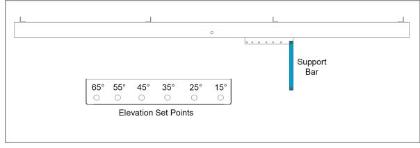
B. Tilt the rack to the desired elevation angle (15°, 25°, 35°, 45°, 55° or 65°) and reinstall the 3/8" hardware securing the Support Bar to the Strong-
