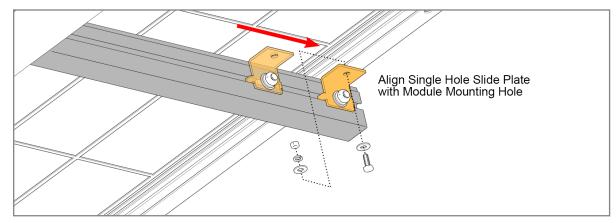
Slide the Single Hole Slide Plates into alignment with Module mounting hole. Secure Module with 1/4" x 3/4" Hex Bolt, Flat Washers, Lock Washer and Hex Nut. Finger tighten for now. Repeat on opposite Rail. Continue in this manner and install the remaining Modules.
