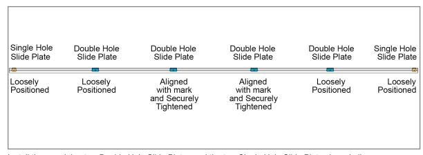
Install the remaining two Double Hole Slide Plates and the two Single Hole Slide Plates in a similar manner, loosely positioning them as shown above. These do not align to any marks or measurements. They will be moved into alignment with the Module mounting holes as the Modules are installed. Hand tighten for now.
