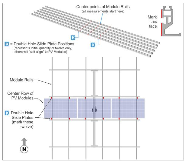
Locate the center of the Rails and mark as shown above. These marks correspond to the "K" dimension representing the locations for the twelve Double Slide Plates (two-per Rail). The remaining Slide Plates do not require marks as they will be aligned to the Module mounting holes as the Modules are installed.
