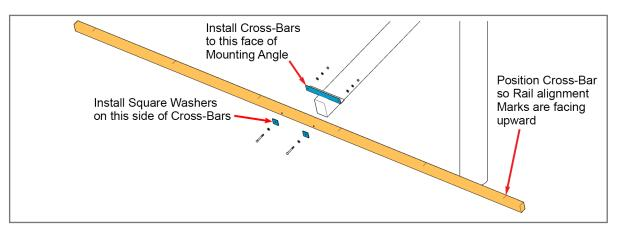
Install the two Cross-Bars with 3/8" x 3-1/4" Hex Bolt, Square Washer, Flat Washers, Lock Washer and Hex Nut. Tighten and **torque to 30-32 ft-lbs.**
