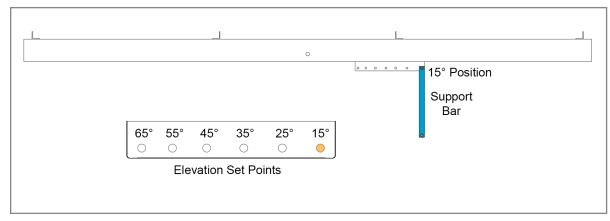
Although this system offers variable elevation set points, for ease of assembly, set the angle to 15°. Optimum tilt setting of the rack will take place later in these instructions.
