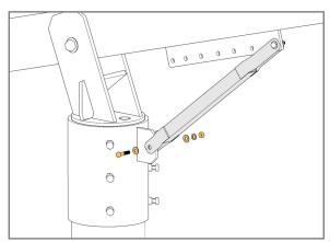
Torque Support Bar hardware at 72-80 ft.-lbs.
