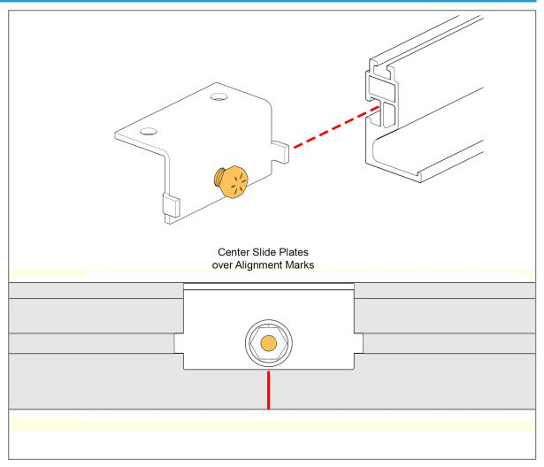
On each of the six Rails, install the two Double Hole Slide Plates to be centered over the previously made marks on the Rails. Insert the head of the Hex Bolt into the Rail channel as shown and align their centers over the marks. Tighten these twelve Slide Plates securely and **torque at 32-34 ft.-lbs.**
