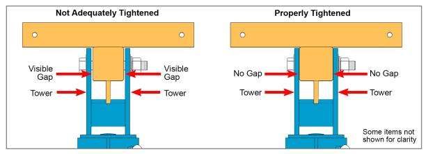
Tighten Pivot Bolt closing any visible gaps between the Strongback and the Mounting Sleeve Towers. **Torque to 330-350 ft.-lbs.**
