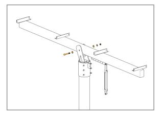
Secure Strongback to Mounting Sleeve with Pivot Bolt, two Flat Washers, Lock Washer and Nut. Secure Support Bar to Mounting Sleeve with 1/2" x 1-3/4" Bolt, two Flat Washers, Lock Washer and Nut.
