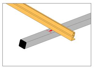
Align the Rail to the alignment marks and straddle its mounting holes over the Cross-Bar. Secure with 3/8" x 2" x 2-5/8" U-Bolt, Flat Washers, Lock Washers and
