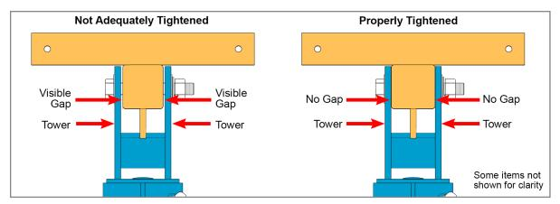
C. Re-tighten the Pivot Bolt. The Pivot Bolt cannot be left loose - the Mounting Sleeve Vertical Towers must be firmly clamped to the sides of the Strongback eliminating any gaps between the Vertical
