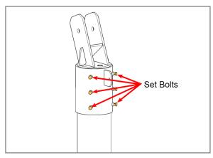
Pivot Tab is pointing north and the Strongback Vertical Towers are leaning south. Tighten Set Bolts and torque to 55-60 ft-lbs.
