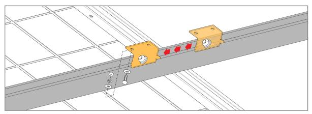
Slide the next Double Hole Slide Plate into alignment with the Module mounting hole. Secure Module with 1/4" x 3/4" Hex Bolt, Flat Washers, Lock Washer and Hex Nut. Finger tighten for now. Repeat on opposite Rail.
