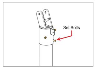
Pivot Tab is pointing north and the Strongback Vertical Towers are leaning south. Tighten Set Bolts and **torque to 32-34 ft-lbs.**
