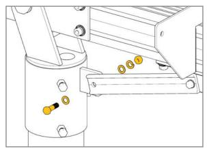
Secure Support Bar to Mounting Sleeve with 3/8" x 1-1/4" Bolt, two Flat Washers, Lock Washer and Nut. Securely tighten hardware to hold structure in place while continuing assembly.
