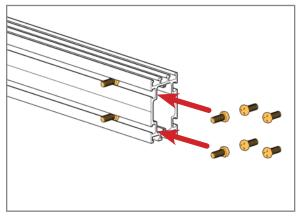
On both sides of the Strongback, insert four 3/8" x 1" Bolts into channels. Arrange Bolts as shown. Align large center hole of Pivot Plates with Pivot Hole of
