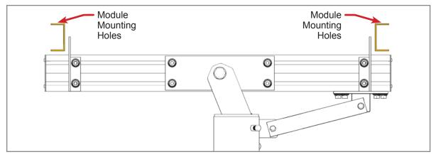
The Module Rails must be oriented and installed to the Rail Brackets as shown above. Ensure that the mounting holes for the Modules are directed upward and in position for installing the Modules.
