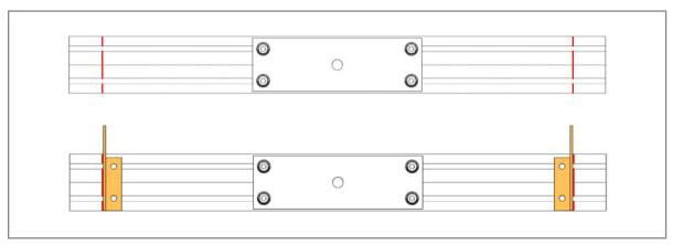
Rail Guide alignment marks (shown in red above for clarity) have been marked-off at the factory. The marks position the span between the Rail's Guides to
