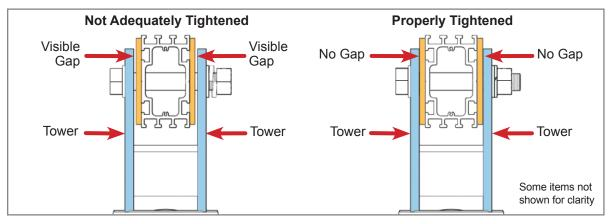
Tighten the Pivot Bolt closing any visible gaps between the Pivot Plates and the Mounting Sleeve Towers. **Torque to 125-150 ft.-lbs.**
