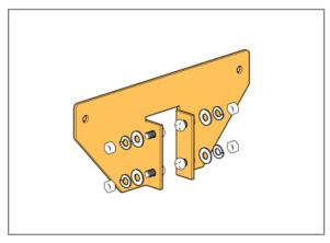
On the two Rail Brackets, loosely install four 3/8" x 1" Bolts, Nuts, Lock Washers, & Flat Washers.
