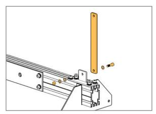
it approximately 1/2" from the end of the Strongback. Attach the Support Bar using a 3/8" x 1-1/4" Bolt, two Flat Washers, a Lock Washer and a 3/8" Nut.
