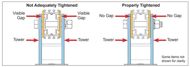
C. Re-tighten the Pivot Bolt. The Pivot Bolt cannot be left loose - the Mounting Sleeve Vertical Towers must be firmly clamped to the sides of the Strongback eliminating any gaps between the Vertical
