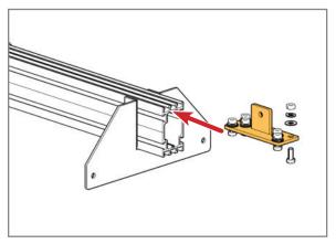
Loosely install the six 3/8" x 1" Bolts, Nuts, Lock Washers, & Flat Washers into the Support Bar Tab. Slide Support Bar Tab onto the Strongback, offsetting
