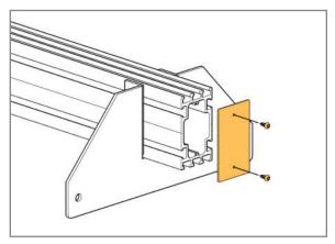
Install one End Cap on each end of the Strongback. Secure with two #8-15 x 1/2" Square Drive Screws.
