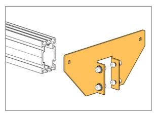
Align Bolts as shown and guide them into the channels of the Strongback. Slide the Rail Brackets to their alignment marks. Tighten and **torque 32-34 ft.-lbs.**
