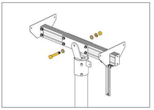
Secure Strongback to Mounting Sleeve with Pivot Bolt, two Flat Washers, Lock Washer and Nut. For now, finger tighten to allow movement during the next sten
