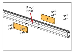
Strongback (inserting Pivot Bolt through the Plates and hole helps with alignment). Secure with 3/8" Nuts, Lock Washers, & Flat Washers. **Torque to 32-34 ft.-lbs.**
