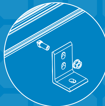
INTEGRATED BONDING MICROINVERTER MOUNT w/ WIRE MANAGEMENT
