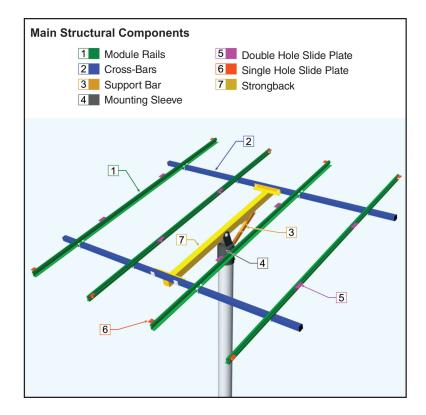
\*PV Modules without a bottom flange and 1/4" mounting holes cannot be used with UPTM's.
