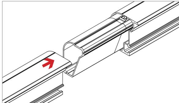
**JOIN TRIMRAIL SECTIONS AT SPLICE:**
