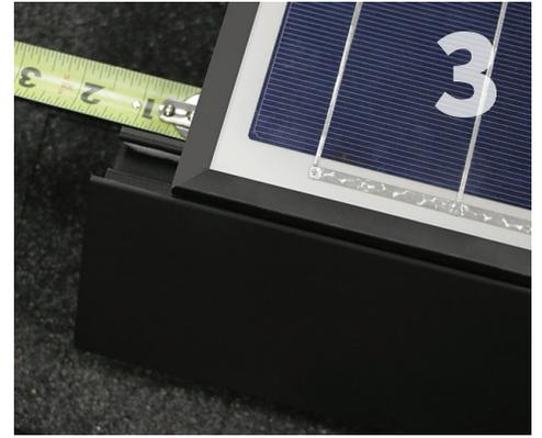
The QSkirt must extend a minimum of 1.2 inches past the edge of the module frame at the outermost corners of the array.
