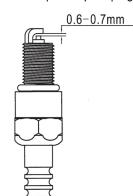
Standard Spark Plug: E6TC/E6RTC/BPR6HS
