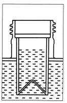
Do not overfill the fuel tank. Provide space for fuel expansion.
