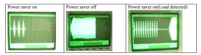
Note: The minimum power of a load to take inverter out of sleep mode (Power Saver On) is 25 Watts.
