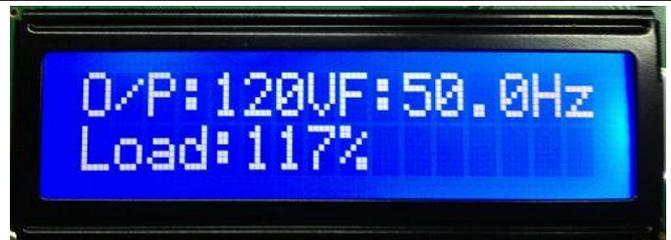
Output Voltage/Frequency and Output Current( in percentage) in Inverter mode
