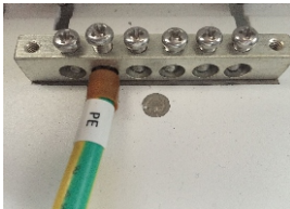
▲ Figure 4.10 Grounding Terminal on Heat-Sink
