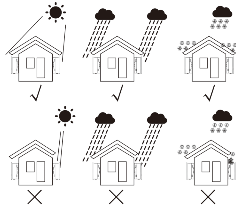
Figure 4.1 Recommended Installation Locations
